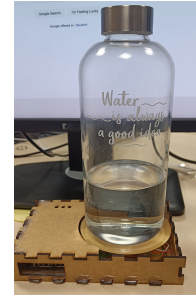
Fig. 3. H2Office gauge system at the in-situ settings
